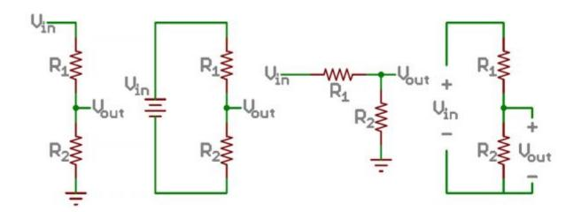
$$V_{out} = V_{in} \cdot \frac{R_2}{R_1 + R_2}$$
